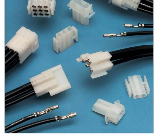
The UL recognized .140 MATE-N-LOK connectors with 3.5 mm diameter pins and sockets, have a 25 A current carrying capacity and are capable of accepting wire with insulation diameters up to 4.5 mm. Both pins and sockets are equipped with dual locking lances, which assure positive contact retention when installed in the housings.
