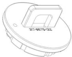
Locking tool for 19-way plug connectors
